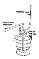
Remove attachment from transmission and elevate the hose higher than the tank. Open the valve, and let any remaining oil return to the tank.
