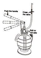
When finished, close the valve as shown in the above diagram.
