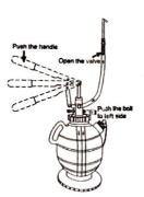
When the handle becomes hard to pump, the fluid is almost full. Push the flow control bolt to the **Left** side and slowly finish dispensing.
