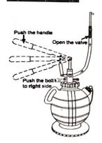
Open the valve and push the flow control bolt to the Right, and pump handle to commence filling.
