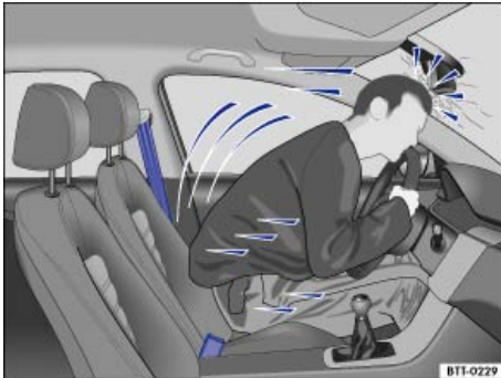
Fig. 51 The unbelted driver is thrown forward.
