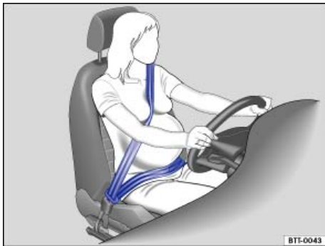
Fig. 57 Proper safety belt positioning for expectant mothers.
