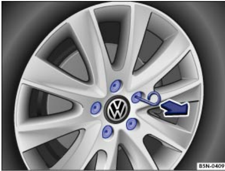
Fig. 177 Pulling cover caps off wheel bolts.
