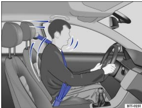
Fig. 53 Belted driver secured by the correctly worn safety belt in the event of a sudden braking maneuver.
