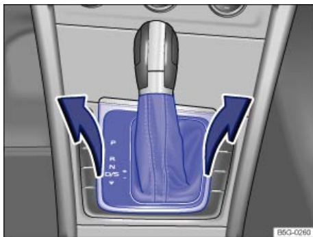
Fig. 171 Removing the selector gate cover.
