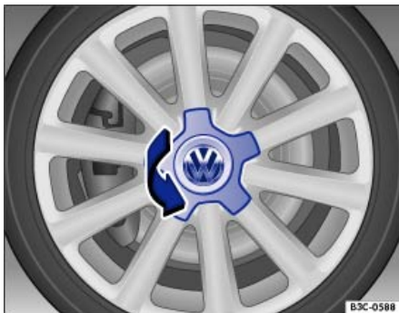
Fig. 176 Twisting the hubcap off.
