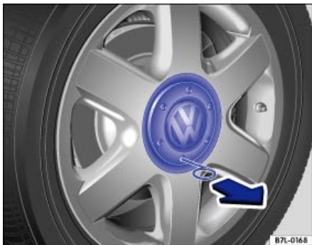
Fig. 175 Pulling the hubcap off.
