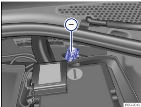
Fig. 188 In the engine compartment: Negative jump-start terminal -
