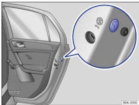
Fig. 167 On the front side of the right rear door: Manual lock, covered by a rubber seal.
