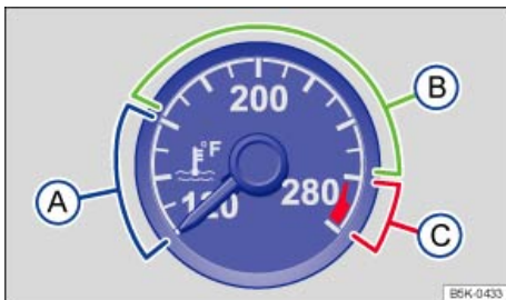
Fig. 158 Engine coolant temperature gauge in the instrument cluster: A Engine cold; B Normal temperature range; C Warning zone.
