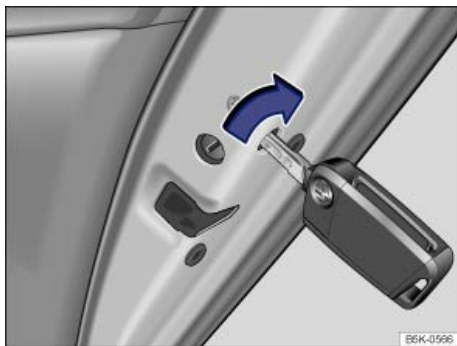
Fig. 168 On the front side of the right rear door: Locking the vehicle with the key bit in the vehicle key.
