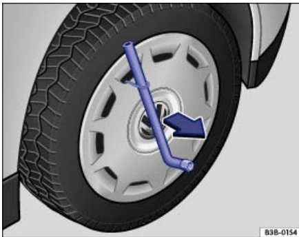
Fig. 178 Pulling the wheel cover off.
