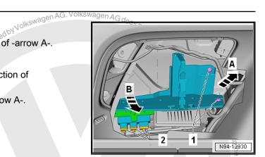
Lift up the Towing Recognition Control Module - J345- -2- and remove in the direction of the arrow -B-.
