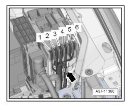
Release the retainers -1, 2 and 4- in direction of -arrow-, remove the Fuse Panel B - SB- -3- and set it aside.
