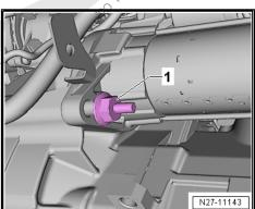
Slide the cap -1- in the direction of the arrow in direction of
