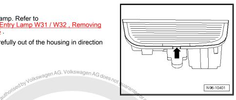
Remove the bulb -1- straight out of the socket.
