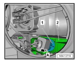
Release and disconnect the connector -1- on the Left Front Turn Signal Bulb - M5- with the bulb socket -2-.
