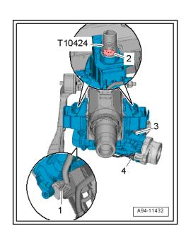
Tighten the new bolts -arrows- until the head shears off.
