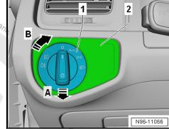
Remove the Rotary Light Switch - EX1- -1-.
