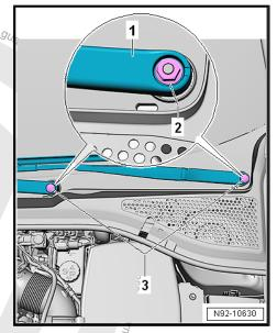
Remove the nut completely and remove the windshield wiper arm -1-.
