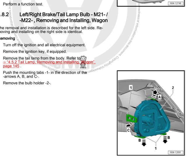
Remove the brake and tail lamp bulb -1- in the direction of the -arrow A- from the bulb holder.
