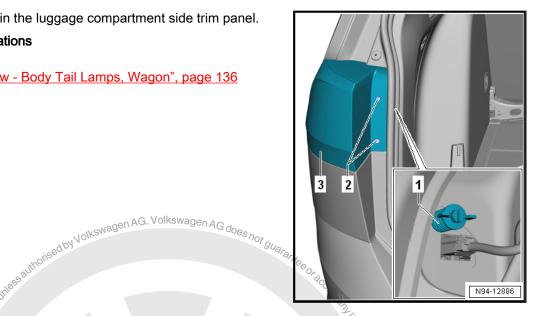
4.5 Tail Lamp, Removing and Installing
