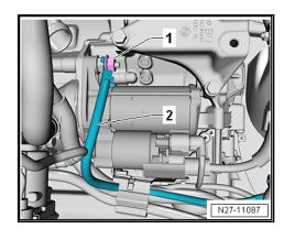
Remove the Starter - B- -3- upward.
