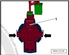
Release the connection -1- and remove and remove the Rain/ Light Recognition Sensor - G397- -2-.
