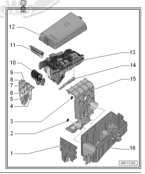
ling. Refer to ⇒ "1.3.2 Fuse Panel A SA, Removing and Installing", page 293.
