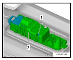
Press the catches -1- and tilt the interior lamp out of the bracket So Stilled unless authorised by Volkswagen AG. Volkswagen AG does not guar -2-.
