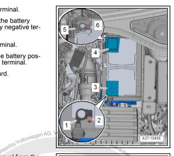
Remove the Battery - A- -3- in the direction of travel from the battery tray and lift it upward out of the engine compartment.
