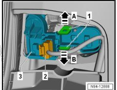
Remove the tail lamp bulb -1- from the bulb holder -2-.
