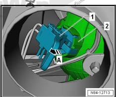
Remove the Left Front Turn Signal Bulb - M5- -2- from the socket -1-.
