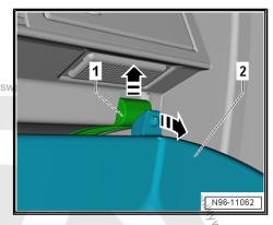
Remove the Glove Compartment Lamp Switch - E26- in the damper -1- from the mount in the direction of the -arrow A-.
