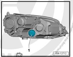
the ret Remove the socket with bulb socket -1- from the reflector -2-Protectedb in the direction of the -arrow A-.
