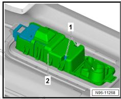
Also use a 3409-, if necessary, to pry the lamp -1- out of the Protected by copying to: 19 - 4. bracket -arrow-.
