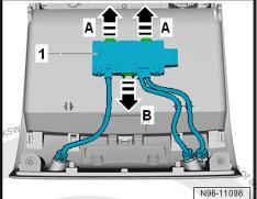
Remove the individual sensor -1- from the roof module.
