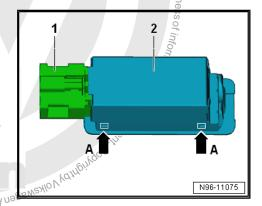
Too Briting State of Remove the bulb -1- from the bulb socket -2- on the back of the glove compartment lamp.
