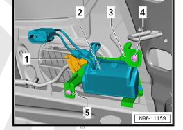
Remove the Converter with Socket, 12 V-230 V - U13--1- from the bracket -2-.
