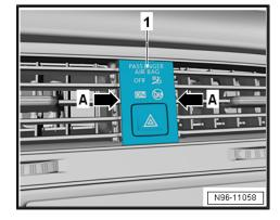
Push the Emergency Flasher Switch - EX3- -2- out of the Front Passenger Airbag -Disabled- Indicator Lamp - K145- in the direction of the -arrow A-.
