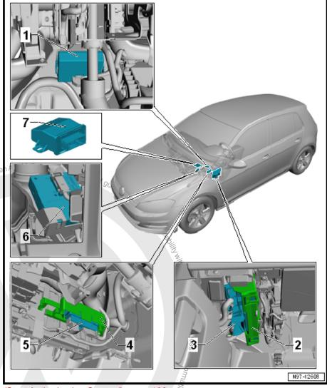
7 - Headlamp Range Control Module - J431- / Cornering Lamp and Headlamp Range Control Module - J745-
