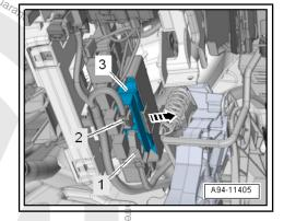
To do this push the tab -1-, pivot the retaining bracket in the direction of -arrow- and remove the connector.
