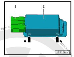
Remove the tubular bulb -2- out of the bulb socket.
