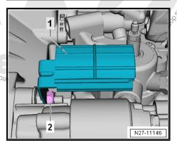
Remove the Starter - B- -2- upward from the vehicle.
