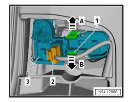
Remove the rear fog lamp bulb -2- from the bulb holder -1-.
