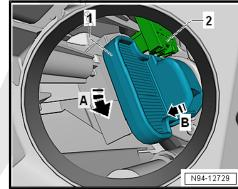
Remove the lamp -2- from the socket -1-.
