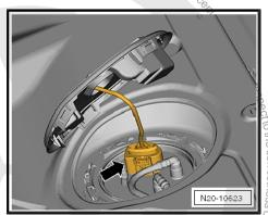
Connect the Vehicle Diagnostic Tester - Test Adapter - 5 Pin - VAS5565- to the connector and to the fuel delivery unit.
