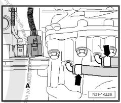
Guide the driveshaft -A- upward and support it in this position with a suitable piece of wood on the tunnel brace -1-.
