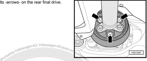
Remove the driveshaft from the centering pins at the rear final drive. Press the driveshaft slightly forward when doing this. Therefore remove the bolts from the center bearing/driveshaft if necessary.
