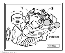
Tighten the bolts -arrows- to the tightening specification. Yolk
