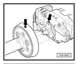
When removing and installing the driveshaft, be careful not to damage the bushing -arrow-.
