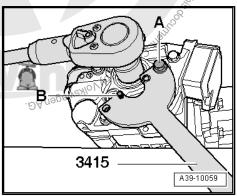
Remove the flange/driveshaft. If difficult use the Puller - Kukko 3 Jaw - 100x100mm - 12/1- .
