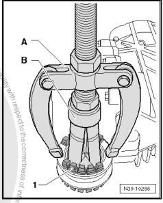
Remove the bonded rubber bushing -1- with a Bearing Installer - Multiple Use - 3348- and plastic mallet.
