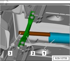
Position the Engine and Gearbox Jack - VAS6931- -1- under the tie rod, and push upward until the driveshaft can be removed from the final drive flange.
