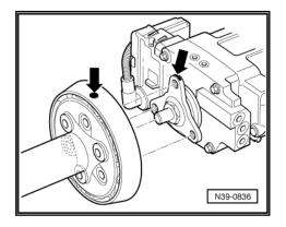
To loosen the driveshaft bolts, counterhold with the Counterhold - Multiple Use - T10172A- and the Counterhold - Kit -Adapter 5 - T10172/5- on the rear final drive.
