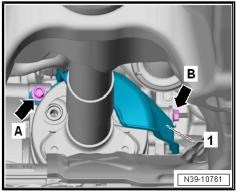
Jen and tig Counterhold the rear final drive to loosen and tighten the driv**hten וווכ** olkswagen AG does not eshaft.
