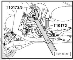
Remove the bolts -arrows- from the intermediate bearing.
