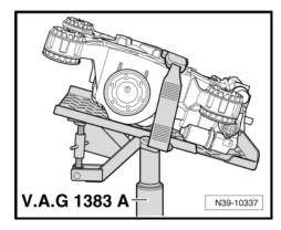
Pay attention that the stop washers -B- are positioned on the rear bearing from above as shown. Correct placement prevents the gummy nipples -A- from falling or sliding out of the washer when installing.
