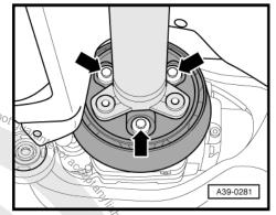
Remove the intermediate bearing -arrows- and if possible, remove the driveshaft to the rear in its fully extended length.
