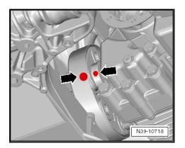
Remove the driveshaft bolts from the front bevel box and the rear final drive -arrows-.
