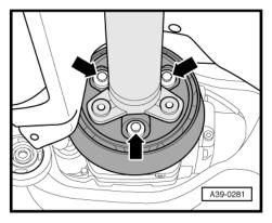
Counterhold using Counterhold - Kit - Multiple Use - T10172-when loosening and tightening the bolts.
