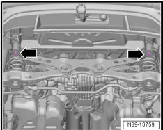
Remove the rear final drive bolts from the rear axle using the Multipoint Socket - T10035- . To remove the bolts the Bits for VAG1331/13 - T10099/1- can also be used.
