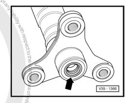
Before removing, see if there is a marking (color dot) on the flexible disc and on the flange/final drive as well as on the flange/driveshaft -arrows-. If the dot is not there, mark the installed position of the flexible disc -arrows-.
