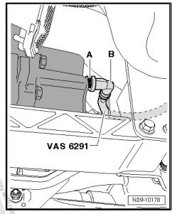
Install the pl. Nm Install the plug -arrow- and tighten. Tightening specification 15
