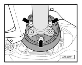
Counterhold using Counterhold - Kit - Multiple when loosening and tightening the bolts: AG does not guarantee of adaptive of a
