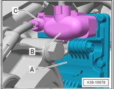
Remove the All Wheel Drive Control Module - J492- bolts -arrows- from the Haldex clutch and the All Wheel Drive Control Module - J492- -A-.
